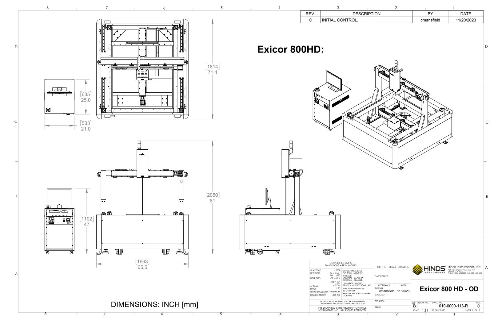
Exicor 800HD: Gantry Max Back Loading Position MAXIMUM GANTRY BACK 1103 43.4 **Max Sample Size** 800mm x 800mm x 500mm
